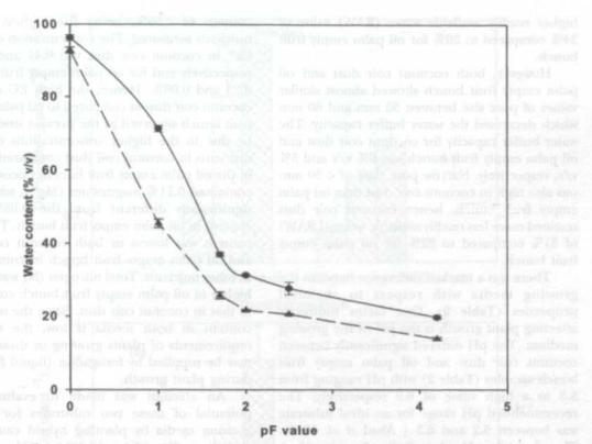
Fig. 1: Moisture characteristic curve for coconut coir dust
